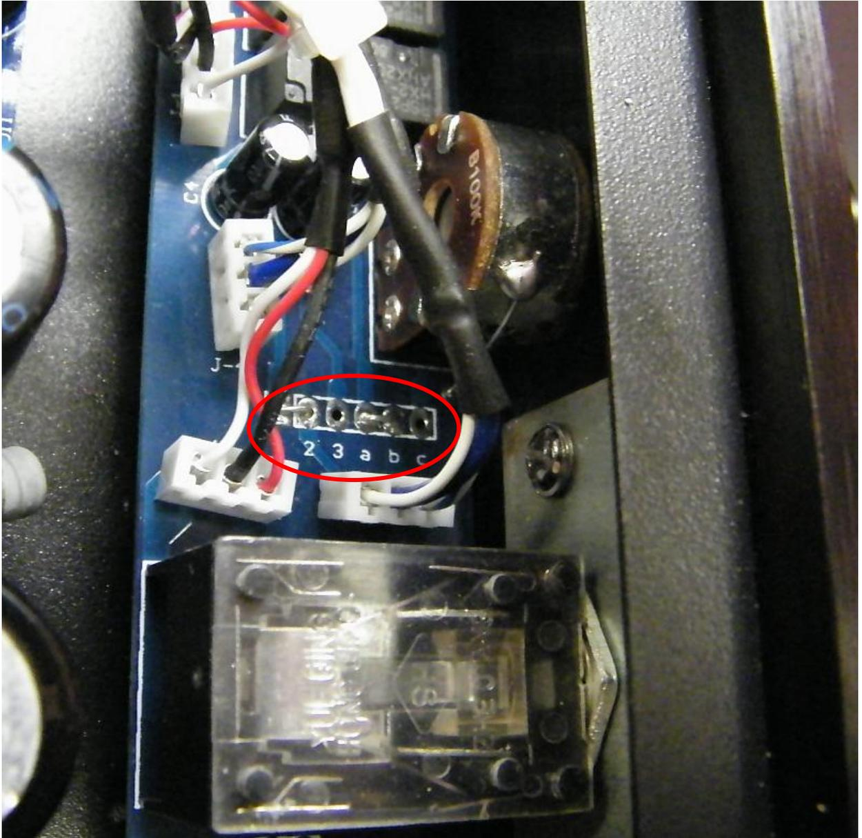
You will need to use a fine tip soldering iron to remove the existing connection wire between 1+2 and a+b. Then you can simply solder 2+3 and b+c together to complete the modification. You don't need to use a connection wire like the factory did – a very small amount of melted solder will connect the position properly. Make sure not to burn the wire around it when you are soldering.
